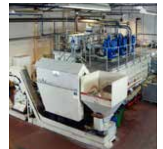
Presses chips from machining into cylindrical briquettes and recovers coolant.
