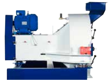
Separates effectively coolant from chips via a high speed centrifuge.
