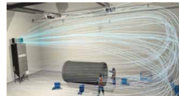
Developed airflow pattern that returns clean air and helps capture fume and contaminants.
