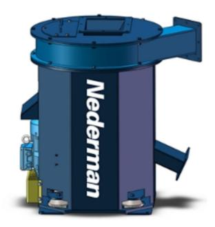
The metal chip wringer type VD40 is a compact-sized chip centrifuge that recovers coolant by centrifuging wet metal chips, while at the same time conveying the dried chips by blowing them to a distant bin.
