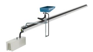
Nederman Waste oil rail is a well covered rail prepared for ventilation to avoid odours in grease pits. High flow funnel and arms secure againts spillage, and is easily adjustable. The rail is mounted with a small incline along the work pit, which makes the waste oil automatically flow to the end of the rail where it is temporarily stored in an 80 litre tank with filter and pump control. The waste oil can then either be drained or be pumped into a central waste oil tank.
