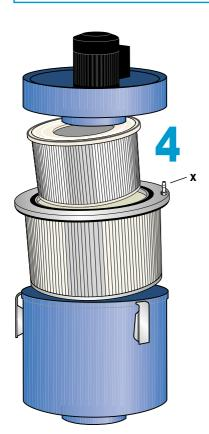
Put the pre-filter, HEPA-filter and fan unit together in the filter unit casing. Important: Make sure that the nipple (x) meets the hole in the filter unit casing.
