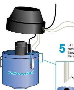
Fit the plastic hoses to the pressure gauge and let them through the cable passage in the top cover.
