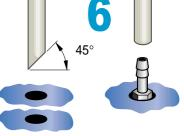
Fit one of the plastic hoses to the nipple. Cut the end of the other plastic hose in a 45° angle. Then push it through the 2 metal sheet holes until it stops against the filter.
