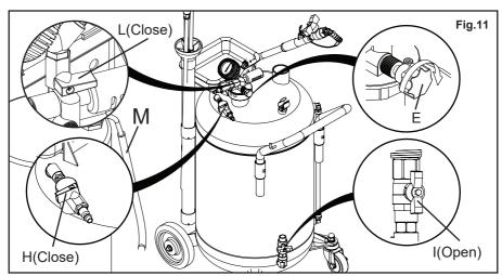
Connect the air supply, and open the valve (H) for draining. (See Fig.12)
