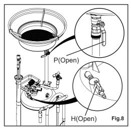
9. Place the oil drainer under the car to collect the waste oil. Turn on the ball valve(P). (See Fig.9)
