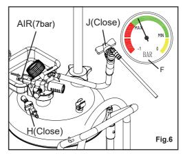
7. Connect the probe (S), then put it into the car engine, turn on the ball valve (J) for sucking oil. (See Fig.7)
