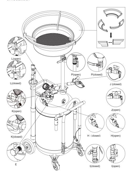
Assemble the handle(B) and the air inlet fitting, turn off the ball valve(H). (See Fig.1)
